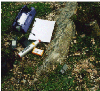
Field basics (Schmidt hammer, GPS, compass, magnetic susceptibility meter)
