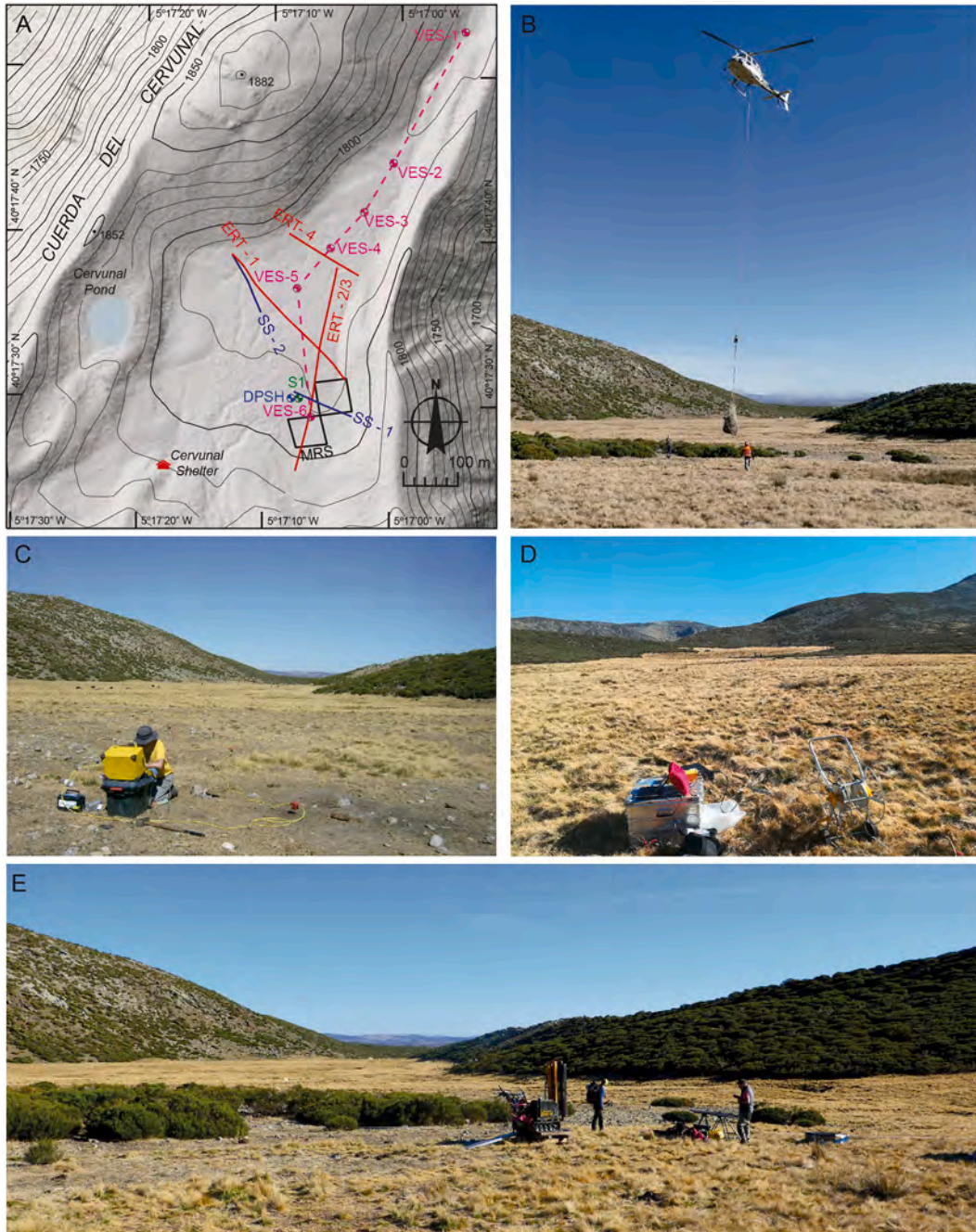
Fig. 2. Field work and data acquisition. A) Geophysical and borehole data location. VES = Vertical Electrical Sounding. SS = Seismic Sounding (Surface Seismic Tomography and Refraction Microtremor). ERT = Electrical Resistivity Tomography. MRS = Magnetic Resonance Sounding. S1 = Borehole. DPSH = Dynamic Probing Super Heavy sounding. Dashed pink line shows the VES pseudo-cross-section of Fig. 5. B) Transportation of the geophysical and borehole equipment by helicopter (the study area is 2–3 h trekking from nearest transitable road by car). C) ERT acquisition. D) SS acquisition. E) S1 Borehole and DPSH test. (For interpretation of the references to colour in this figure legend, the reader is referred to the web version of this article.)
